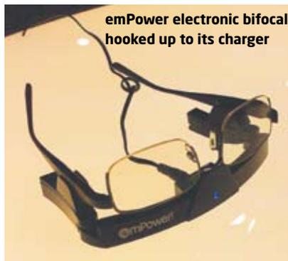
emPower electronic bifocal hooked up to its charger
